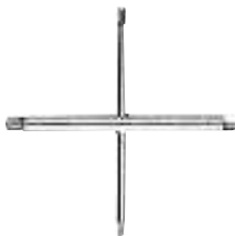
19 053 000 Splined Spider Key Ø 8 x Ø 9 x Ø 13 x Ø 15 To disassemble/assemble the valve seats of concealed valves 1/2" to 3/4" and Grohmix bath- and universal mixer 1/2" and changeable seats of two-lever faucets 3/8" GROHE Long-Life finish
