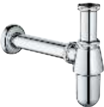
28 920 000 chrome Trap 1 1/4" for basins with fixed dip tube wall connection sliding escutcheon GROHE Long-Life finish
