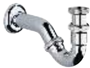
28 946 000 chrome P-trap 1 1/4" for bidet wall connection sliding escutcheon wall support 250 - 265 mm GROHE Long-Life finish
