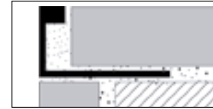
Wall tile corner
